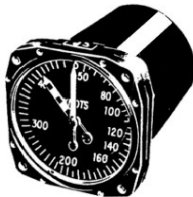
Fig.2.11. Maximum allowable airspeed indicator
