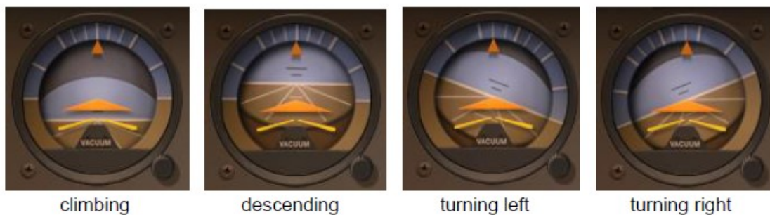
Fig. 3.6. Operation of Attitude indicator
