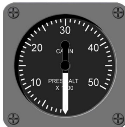
Fig. 5.16 cabin pressure altitude indicator
